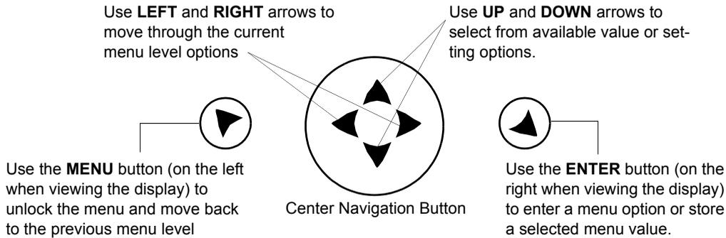
**Note:** *Navigation system buttons' functions invert automatically when the fixture is turned upside down.*
